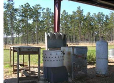
Figure 3. An example of a small processing unit includes the killing cones, a propane tank, a propane-heated scalding machine, the plucker, and a table for evisceration (clockwise from back).
