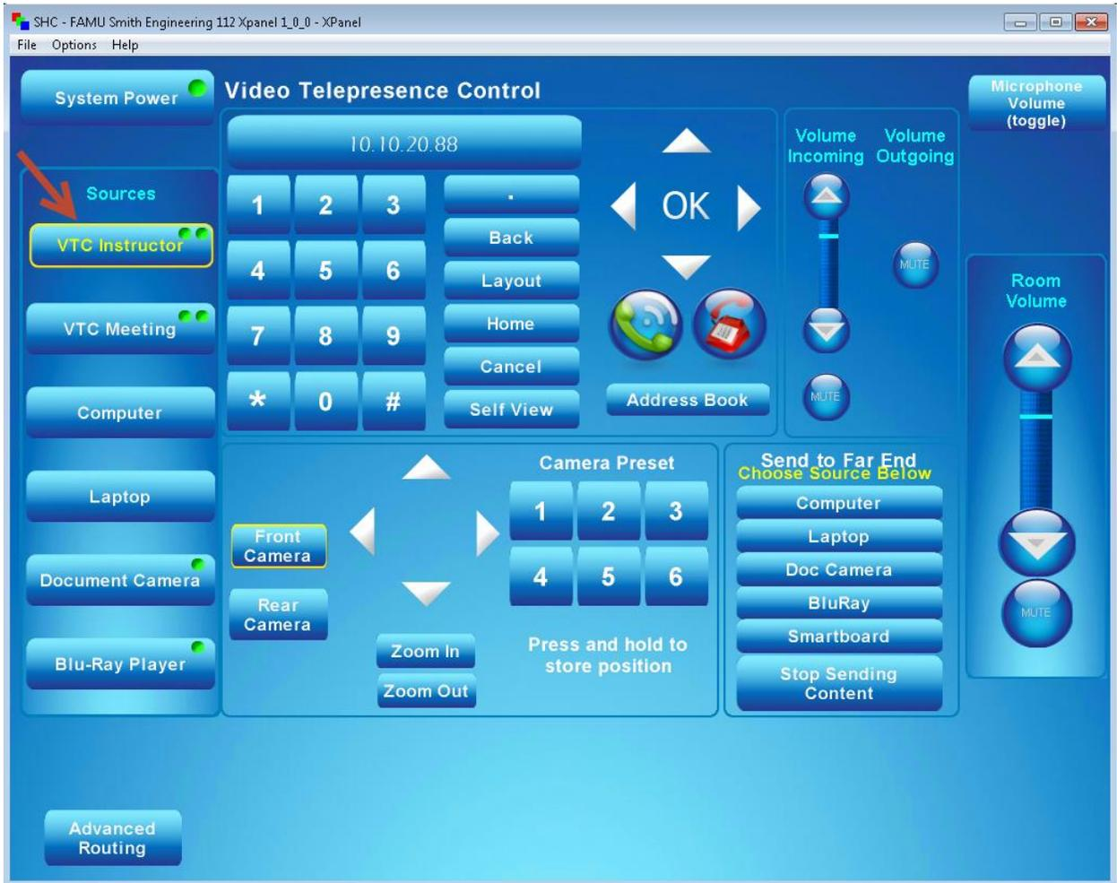
6. Instructors must use the device options on the right of the touch panel underneath the 'Send to Far End' button, to share content with your remote students. Ex: **Computer, Laptop, Document Camera, BluRay, Smartboard.**
