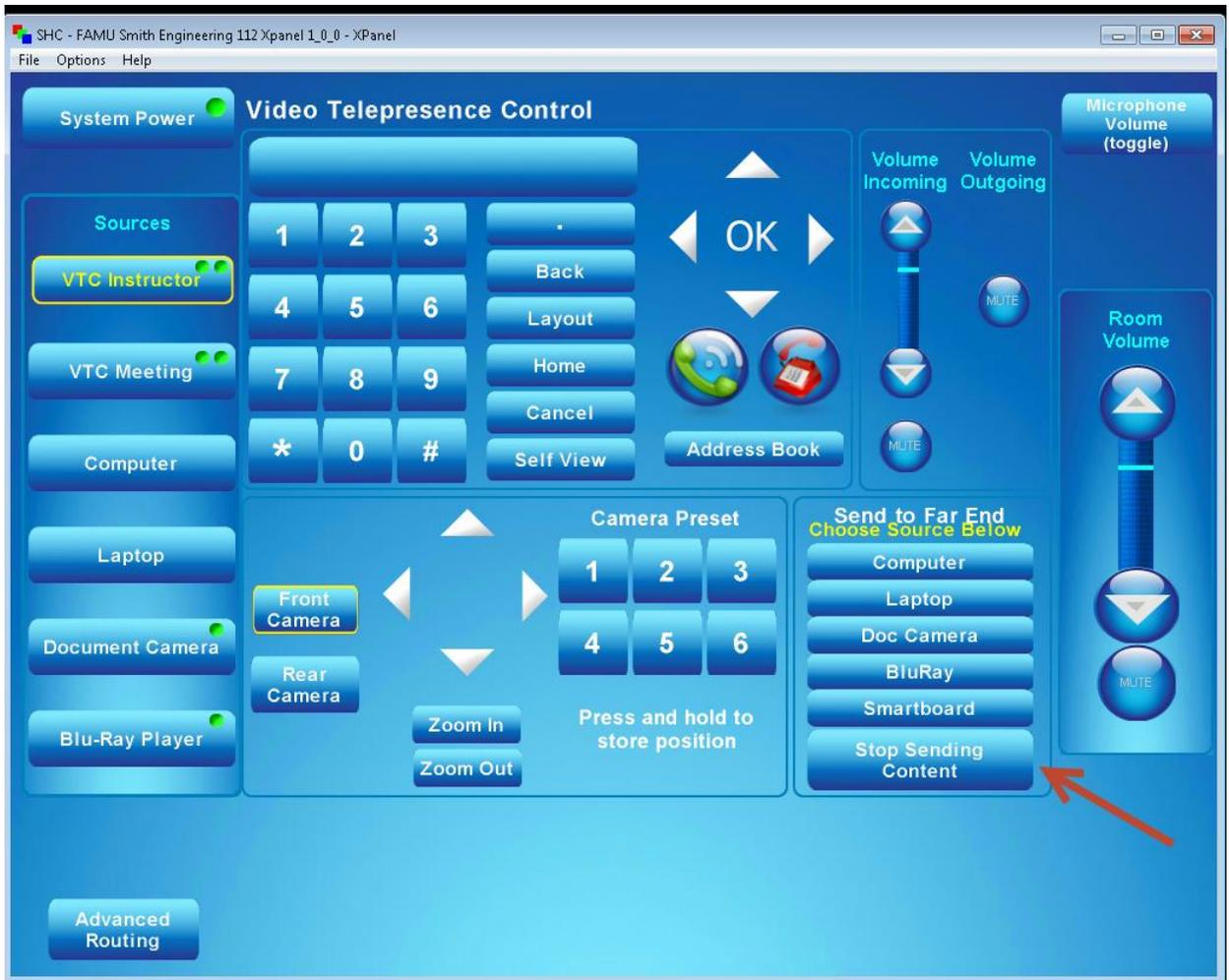
12. The **Stop Sending Content Button** underneath the **Send to Far End** device options is press when control is pass between Presenters' or if a device fail to show content.
