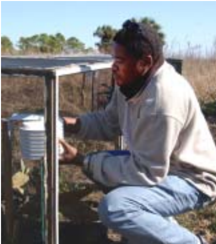
Masters graduate student Stephen Mclean installing temperature data loggers in his experiment cages at St. Marks National Wildlife Refuge, FL.
